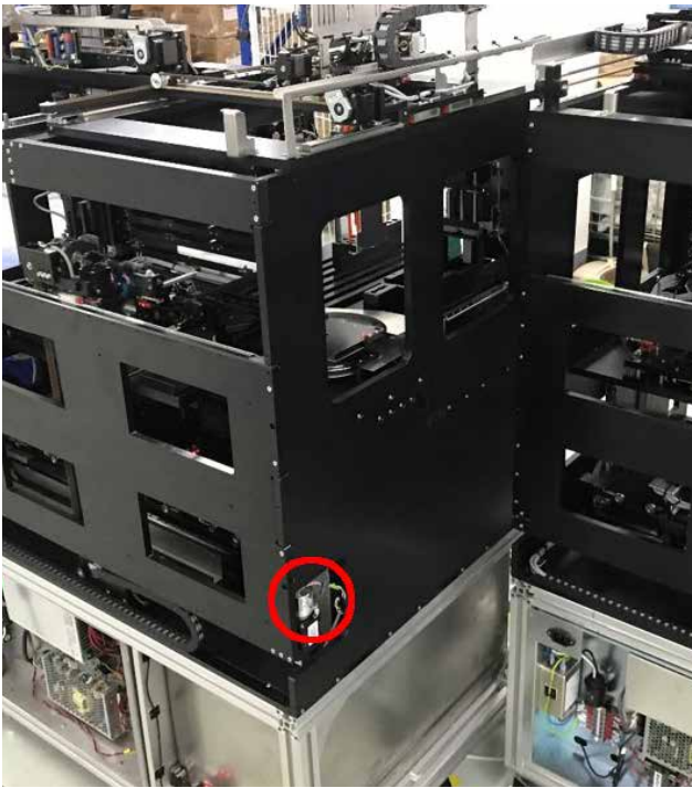
Image 3: Encoder WDGA36 CANopen for the organisation of the carrier plates
