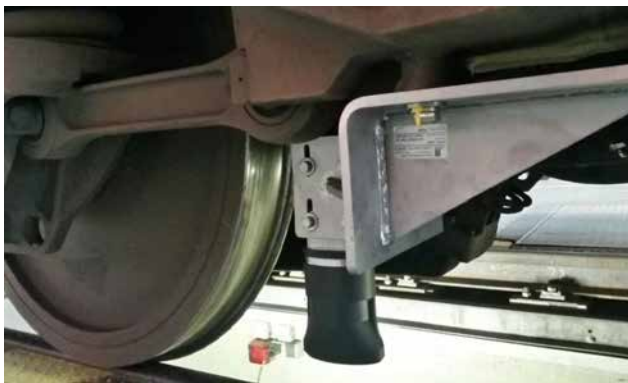
WA2101_1: In Germany, for example, the HaslerRail speed sensor is used on the ICE.
