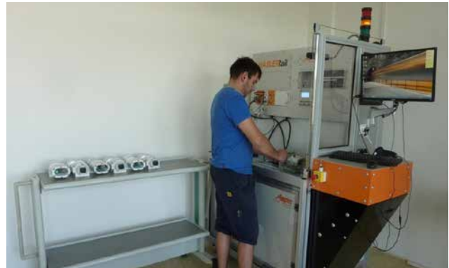
WA2101_3: Calibration of the optical sensor system and final testing.
