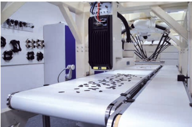
Image WA1601_1a and WA1601_1b Adept Quattro is designed specifically for high-speed handling applications. This depends on very precise measurements – and these are just what is provided by Wachendorff Automation's LMSMA2x/3x length measuring system.
