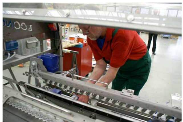
Image 9 Ullrich Dettweiler fits a Wachendorff encoder. The type used here is available with between 2 and 25000 pulses. The customer can also select between the different resolutions, output circuits and connectors.
