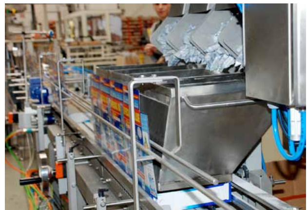
Image 2 85% of the packaging machines are used in the foodstuffs industry. However, folding boxes - Econo-Pak's core business - are also used in other industries. Dishwashing tablets are being packaged here for example.
