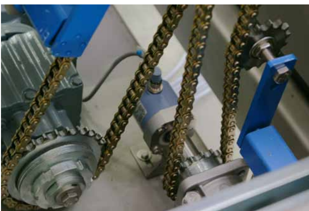
Image 6 Wachendorff encoders determine the exact position of the cardboard packaging. Their impulses provide information to the control on when the next process substep can be triggered.
