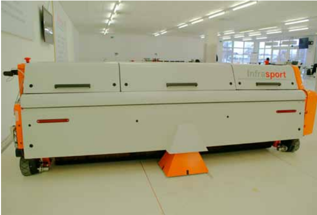
Image 4 The Bodenwart cleans a path 240 centimetres wide, completing the wet cleaning of an entire sports hall in 15 minutes.
