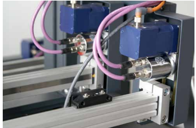
Image 5 Six encoders are needed for this BST solution. Each web has a pair of sensors which record the position and communicate it via the CANopen interface.
