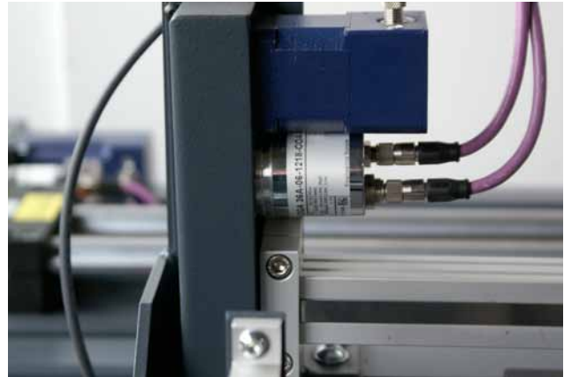
Image 1 The rotary encoder was slightly modified for BST. It now has two connections for special plugs.
