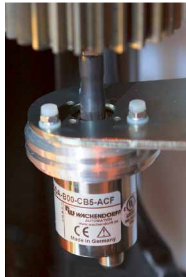
Image 4: Sensors are a prerequisite for automated processes. In picture: WDGA absolute encoder with EnDra® multiturn technology from Wachendorff.
