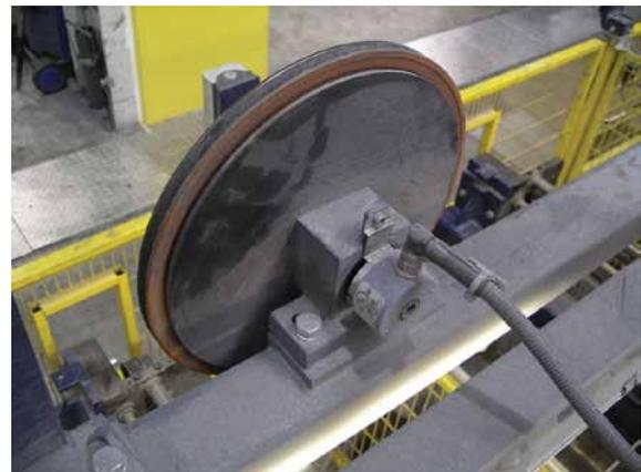
Image 4-5: Since the encoders are totally exposed, they need to be particularly impervious to external influences. No problem for Wachendorff devices, which are extremely robust.
