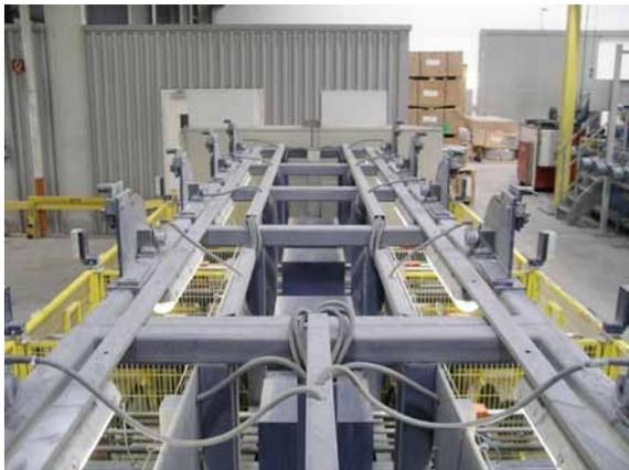
Image 8: Wachendorff encoders measure the exact feedrate to allow precise regulation of the motor drive by the control unit.
