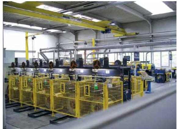
Image 11: Mechanised wire drawing is not feasible without high-performance control equipment.
