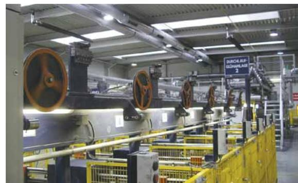
Image 6: Wachendorff encoders ensure that the wire is subjected to the annealing process for a consistent time.
