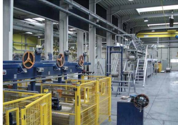
Image 9-10: Once the wire has passed through the annealing unit, it is once more wound onto coils and processed further.
