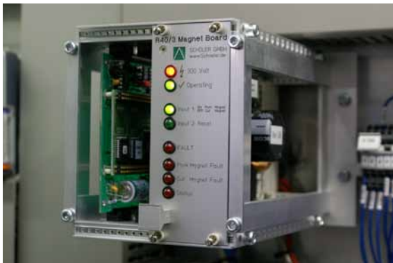
Image 6 Board (Wachendorff): This is where the brains of the tube cutting equipment are located. The controller has been developed by Schöler. Both Wachendorff encoders supply important information.
