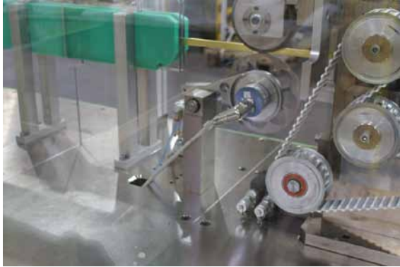
Image 5 Encoder counter (Wachendorff): The second encoder calculates the exact speed of the finished tube in order to determine the exact time of the cut. This ensures that the tube sections have the desired length to the nearest millimetre.
