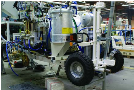
Fig 1: Marking machine for road marking
