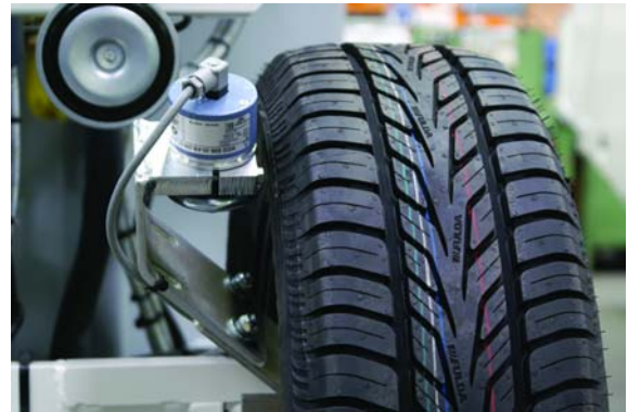
Fig 3: WDG 58B with longer shaft and special bearings
