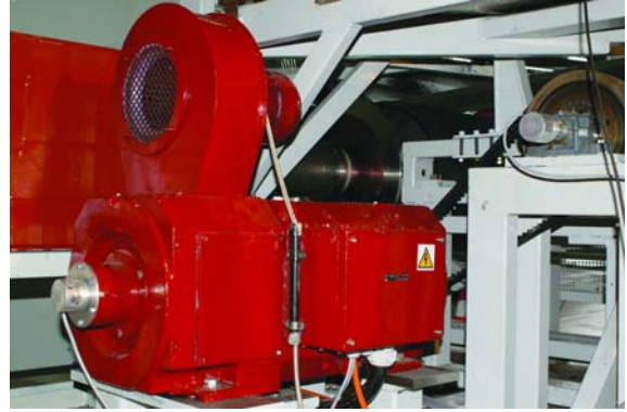
Image 3 The drive for the moving belt is also fitted with a Wachendorff encoder.
