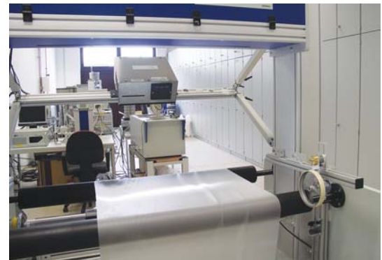
Speed measurement for quality control of films
