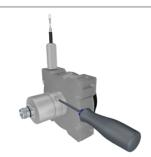
By tightening (approx. 2 Nm) the outer radial screw with a 2.5 mm hex wrench the encoder housing will be clamped to the sensor housing and secured from twisting. The system is now ready to be used.
